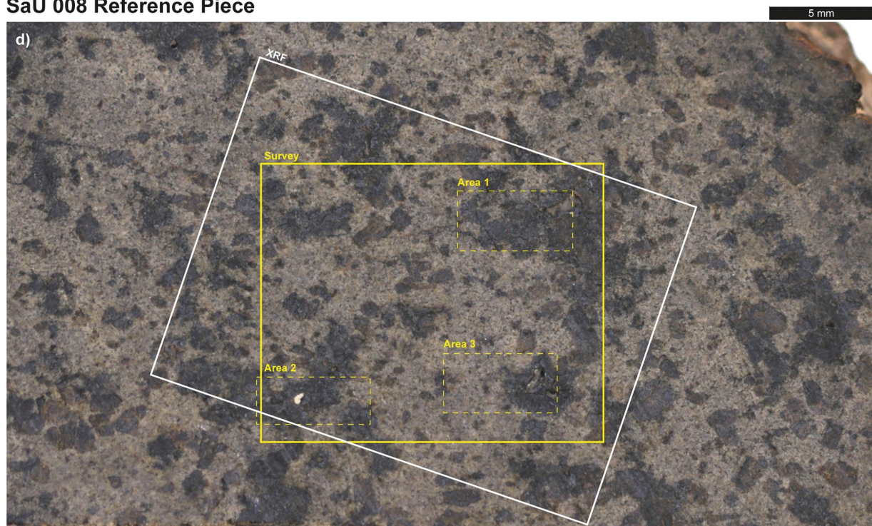
Figure 1. (a) Photograph of the Sayh al Uhaymir (SaU) 008 meteorite calibration target (the flight piece) taken during pre-launch characterization. (b) WATSON image of the flight piece taken on sol 540 of the mission on Mars. (c) The meteorite calibration target as seen by the SHERLOC autofocus context imager (ACI) on sol 545, colorized and illustrated to show footprints of the pre-launch MOBIUS maps (white) and SHERLOC maps (yellow) as of sol 935. (d) Photograph of the SaU 008 reference piece, illustrated to show footprints of X-ray fluorescence (white), DUV fluorescence (solid yellow), and DUV Raman (dashed yellow) maps.
